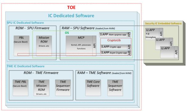
Figure 2: TOE software design decomposition
